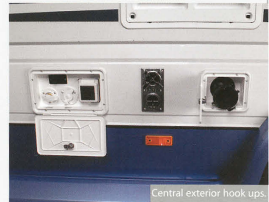
Easy access sewer hook up
