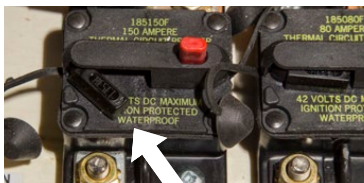
ARM DOWN INDICATES TRIPPED BREAKER
