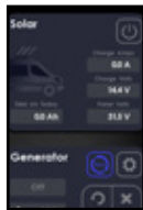
TOUCHSCREEN CONTROL PANEL CONNECTED TO THE MPPT CONTROLLER.
